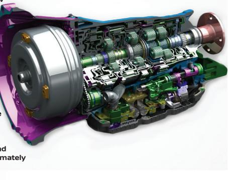
Torque converter lock-up is also accomplished faster, resulting in less slip. The 9-speed can be locked as early as first gear, depending on throttle application and speed. Higher numeric ratios help improve standing start acceleration while close ratio spacing keeps the engine in its optimal power band.
